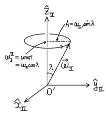
The  $\vec{\omega}_{II}$  vector goes once around in time  $T = \frac{2\pi}{\Omega}$ .
